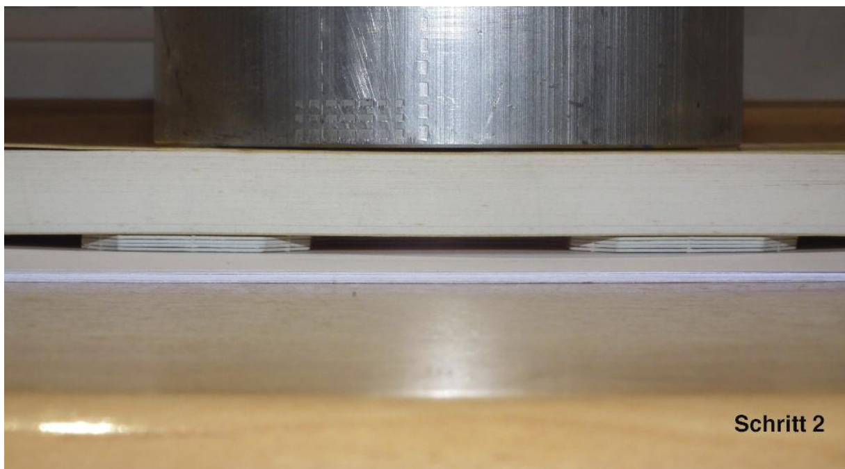
The four parts of the base plate are glued together and pressed during the drying process to prevent the base plate from warping during drying. A plywood board and a weight (e.g. a large piece of metal or books) are helpful for this.
