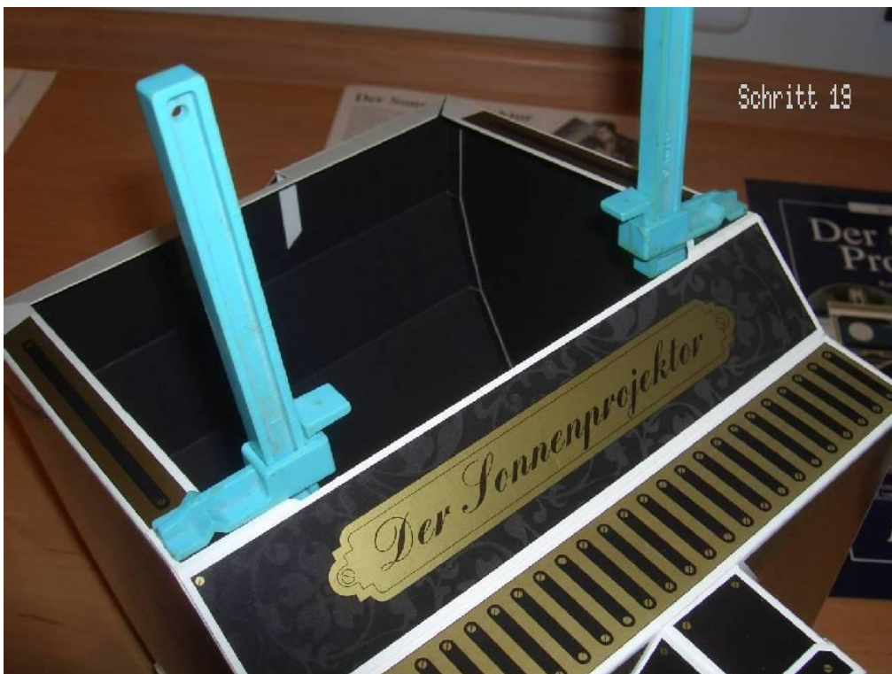
Step 19: Gluing the side flaps of the plane mirror holder (again with the help of mini clamps).
