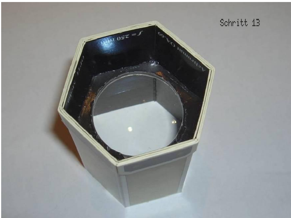
Step 13: Objective tube with the objective lens inserted in its holder. The cuff (step 14) has already been attached before (see above).
