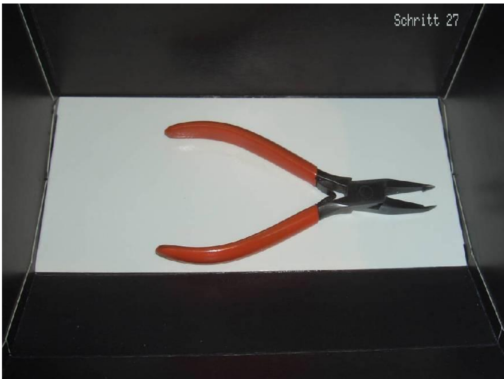
Step 27: Attachment of the projection surface inside the projector. A slight weighting ensures flat adhesion.
