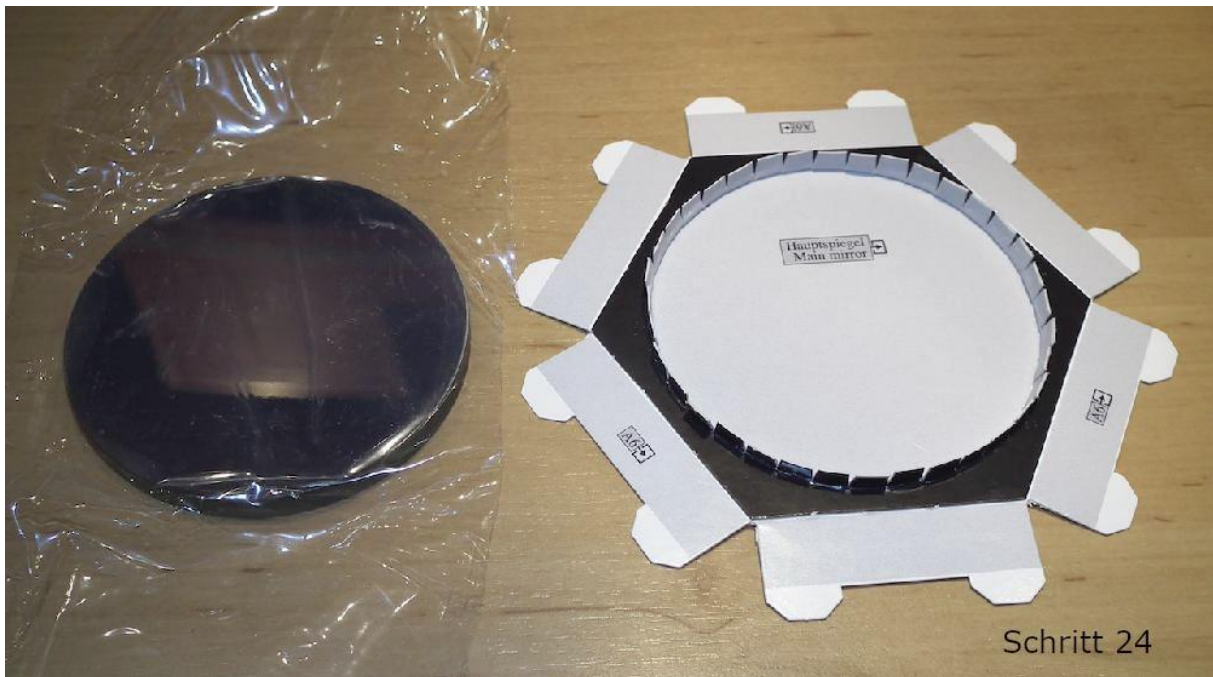
Step 24: Base plate and holder of the main mirror. Contrary to the instructions, the tabs of the base
