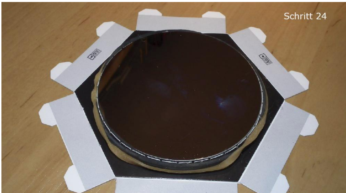
Step 24: Base plate and holder of the main mirror. Contrary to the instructions, the tabs of the base
