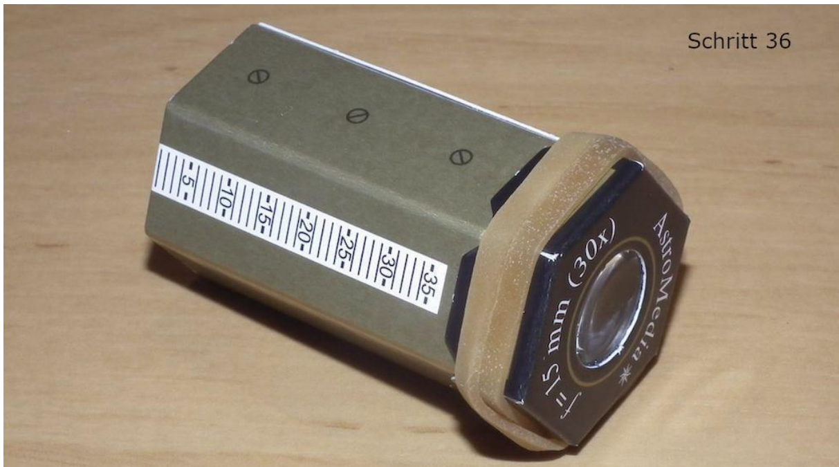
Step 36: The completed Ramsden eyepiece. We will not document the assembly of the Steinheil eyepiece, as the assembly is virtually identical to the principle of the Ramsden eyepiece.
