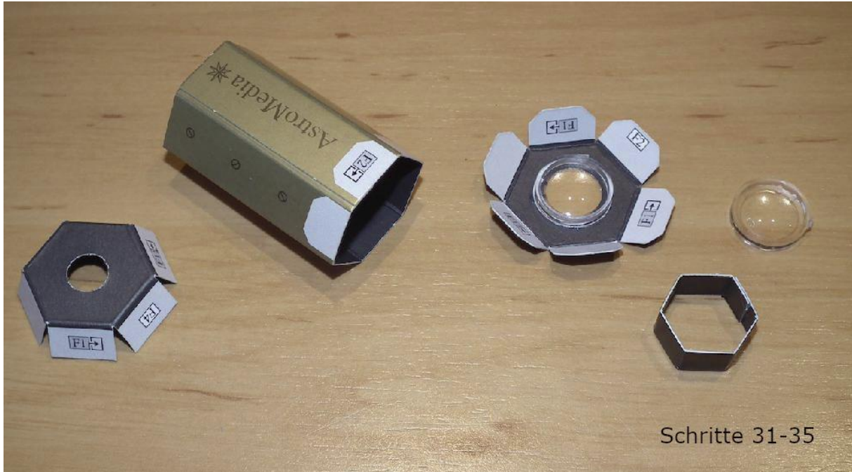
Steps 31 – 35: Partially assembled Ramsden eyepiece. The still loose lens is placed on the lens already glued to the ocular lens holder by means of the hexagonal collar and glued there. The diaphragm on the left of the picture finds its place at the other end of the eyepiece tube.
