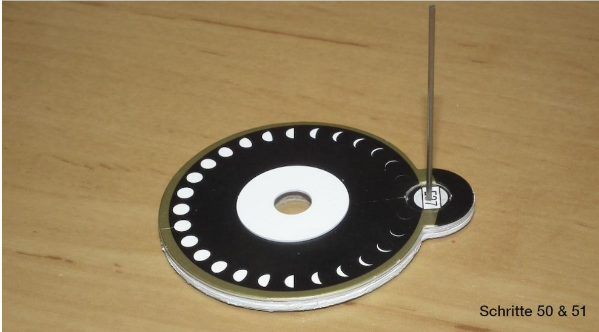
Steps 50 & 51: The moon orbit disc after steps 50 and 51. The metal pin is first removed again and serves here only to check its vertical alignment.
