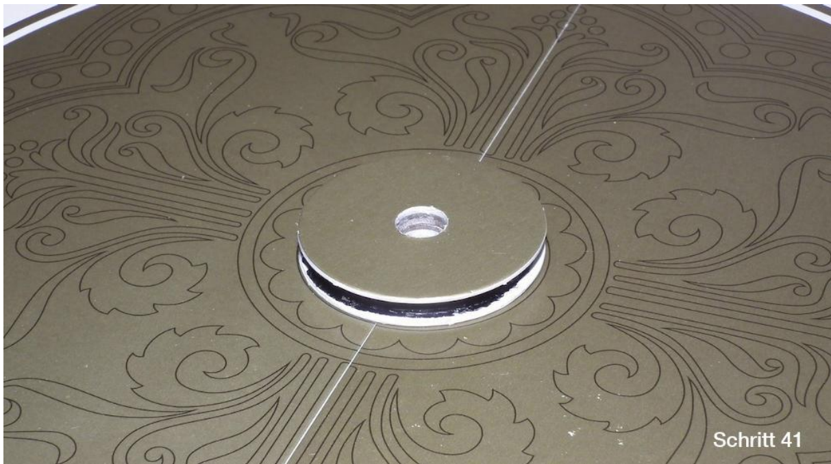
Step 41: Create the earth tilt drive wheel according to step 41 and mount it on the underside of the ecliptic disc.
