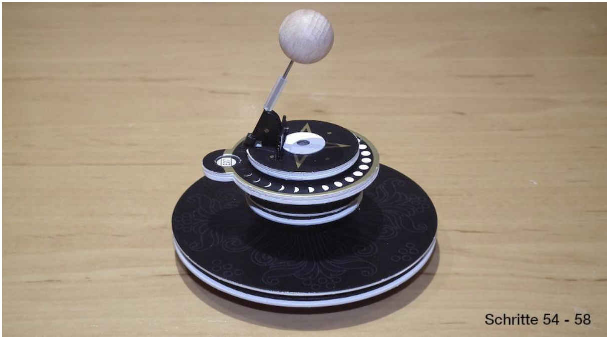
Steps 54 – 58: Earth axis base made in the familiar layered construction method, now with assembled earth axis holder and "earth sphere" attached for testing purposes.
