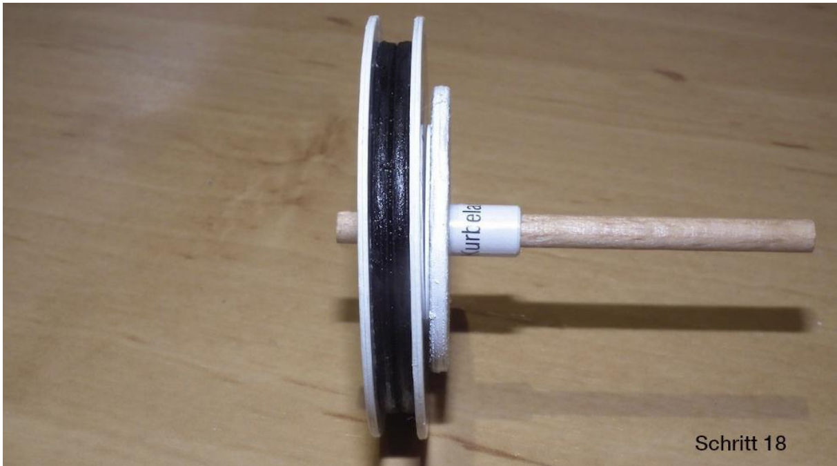
Step 18: Driving wheel with bearing and crankshaft, created according to step 18.
