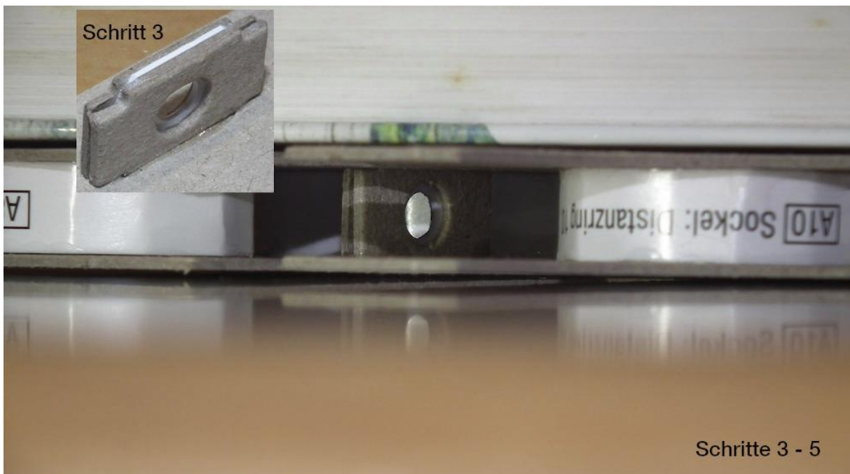
Steps 3 - 5: The small picture detail shows the inner bearing of the crankshaft created in step 3. In steps 4 and 5, the remaining base walls and spacer rings are glued and pressed together.
