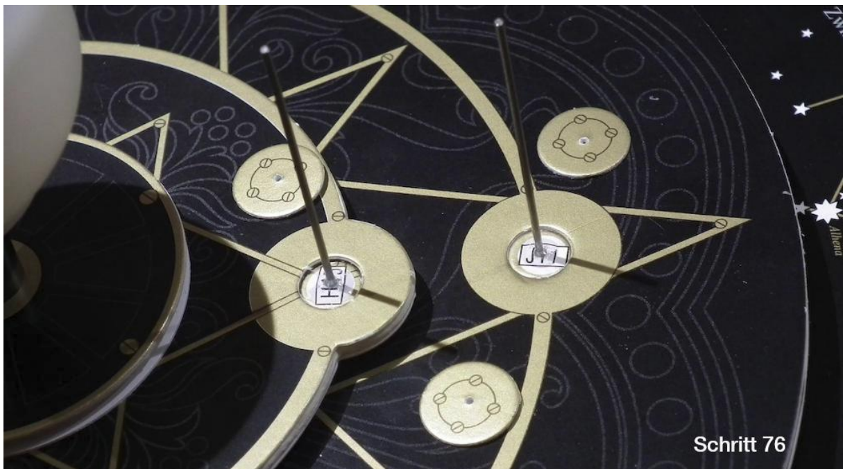
Step 76: Assembly of the pins and covers for Mercury, Venus and the Moon.
