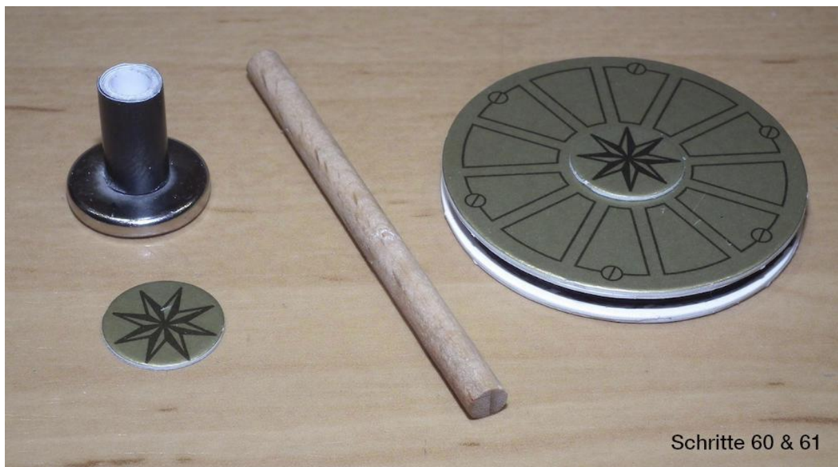
Steps 60 & 61: Magnet with bracket, axle and impeller Earth rotation ready for installation in the planetary gear.
