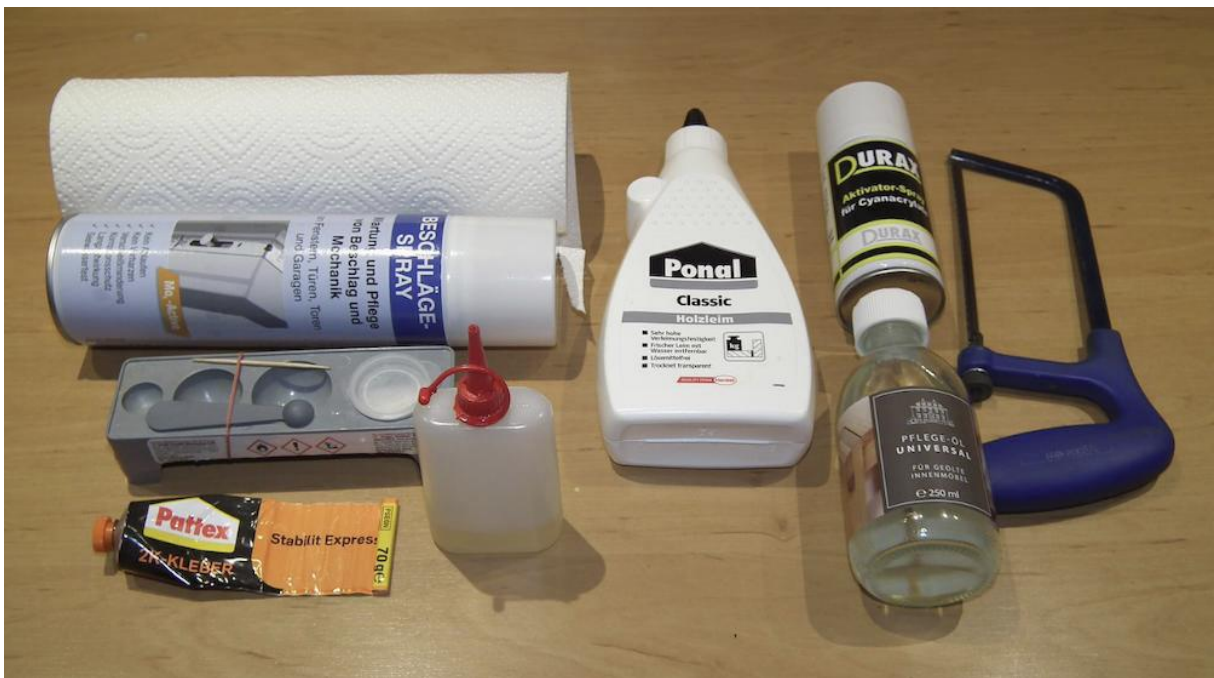
Other useful but not absolutely necessary utensils. Wooden parts should be treated with a furniture care oil before oiling with machine oil, which hardens as a protective layer 1-2 hours after application. Teflon spray can be used as a sliding aid on the inner radii of the bearing washers.
