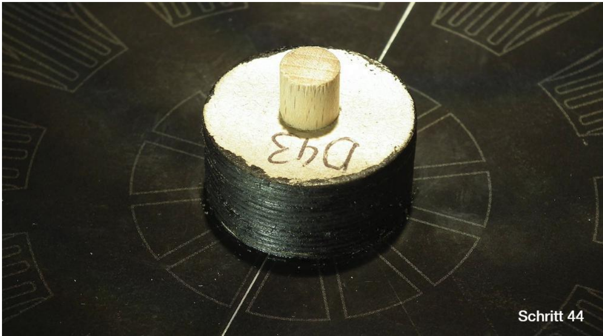
Step 44: The cylindrical block mounted on the top of the ecliptic disc consisting of 14 discs "D43".
