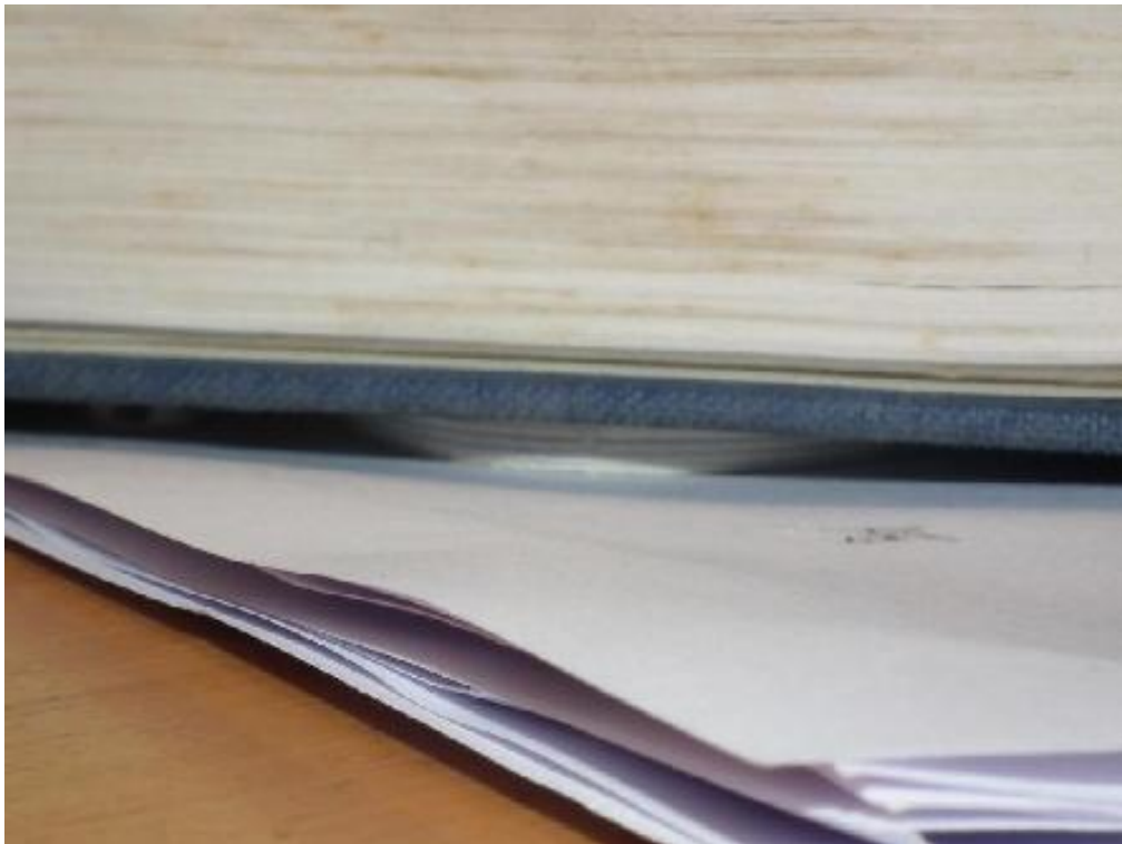
A thick book as a weight to press the glue during the hardening process.
