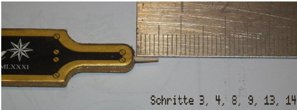
Steps 3, 4, 8, 9, 13, 14: The tip length of the legs must be exactly 5mm. As toothpicks tend to break, it is not advisable to glue them in the legs - it would then be difficult to replace them...if necessary, wrap them with a piece of paper.
