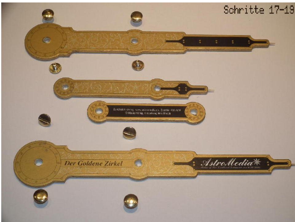
Steps 17 – 19: The legs, the steering bar and the fittings ready for assembly.
