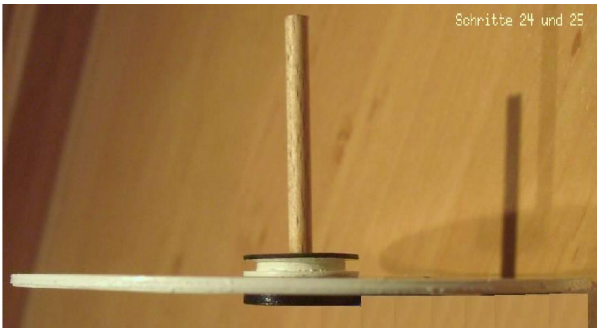
Steps 24 & 25: Side view of the colour disc carrier with shaft, its holder and the impeller.
