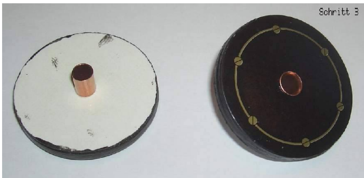
Step 3: After notching the edges of the bearing block, the metal bushes are inserted. The easiest and cleanest way to do this is to use superglue.
