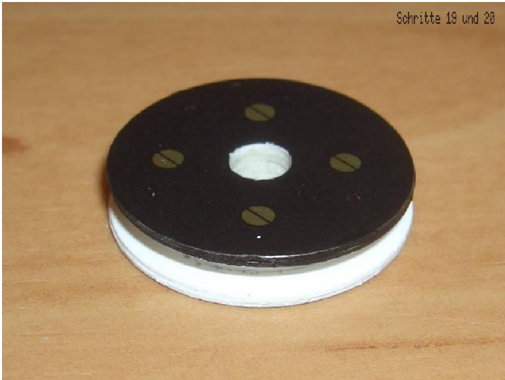
Steps 19 & 20: The impeller consists of 4 inner discs and two upper and two lower guide discs, with edges already dyed to fit.
