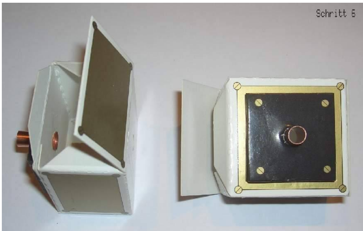
Step 6: Creation of the lower shaft bearings.
