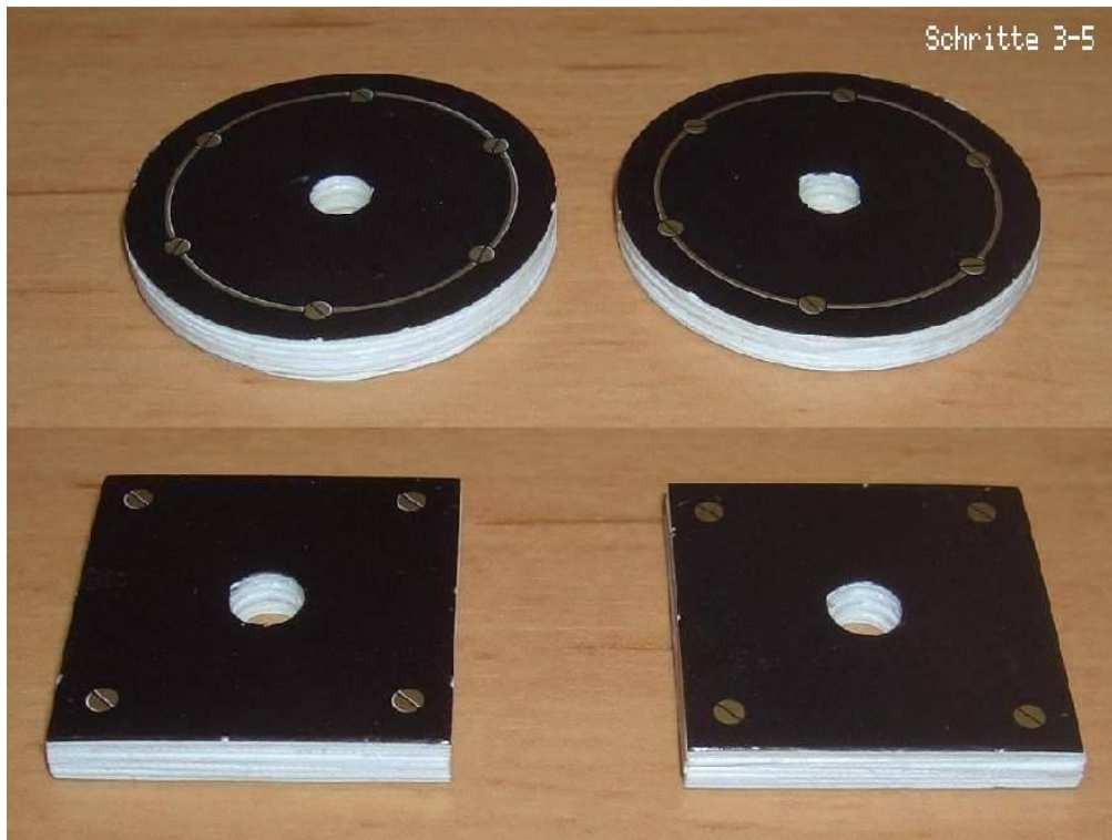
Steps 3 – 5: Gluing the cardboard discs into blocks for the upper and lower shaft bearings.
