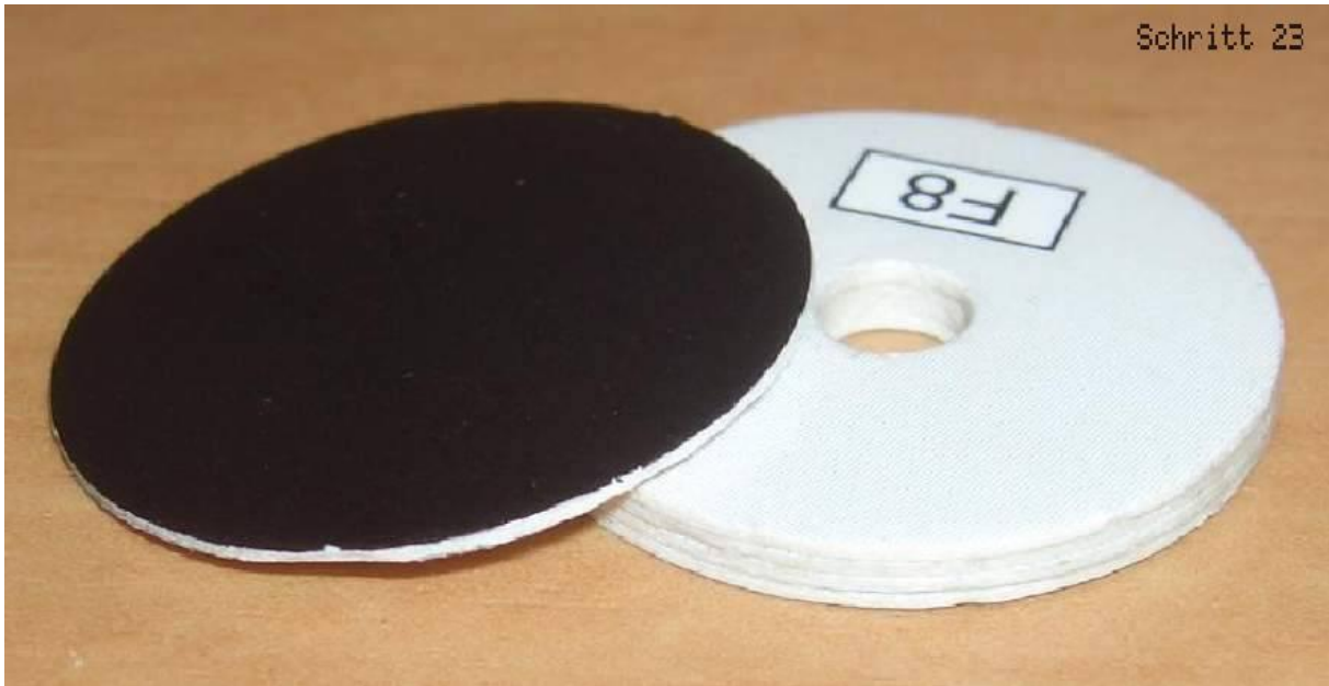
Step 23: The shaft holder block for the colour disc carrier. The black cover is only fitted after the shaft has been inserted.
