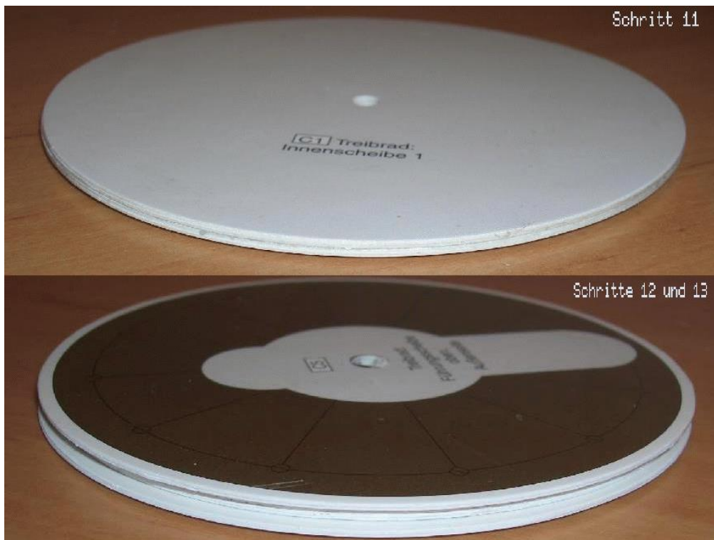
Steps 11 – 13: Creation of the driving wheel consisting of eight discs.
