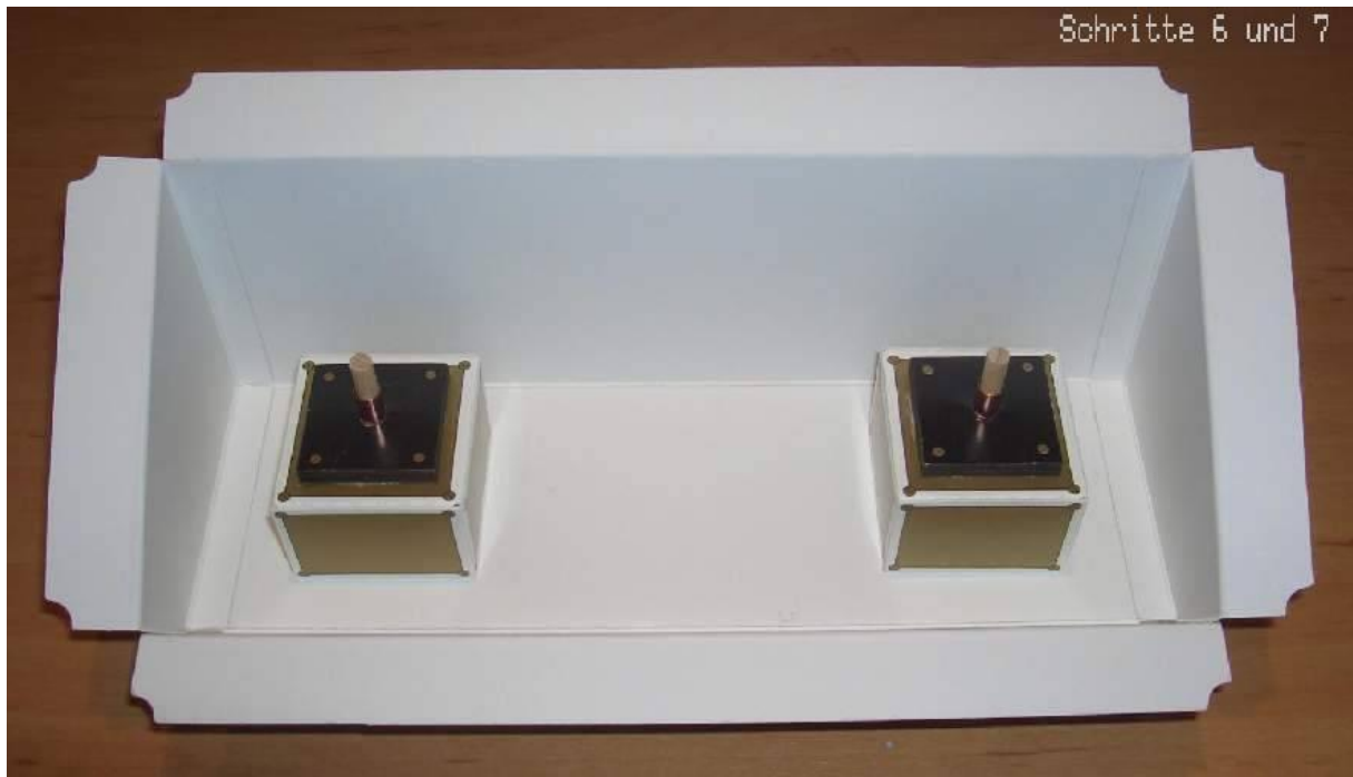
Steps 6 & 7: Gluing the lower shaft bearings to the underside of the desk and checking for lightness of the shafts.
