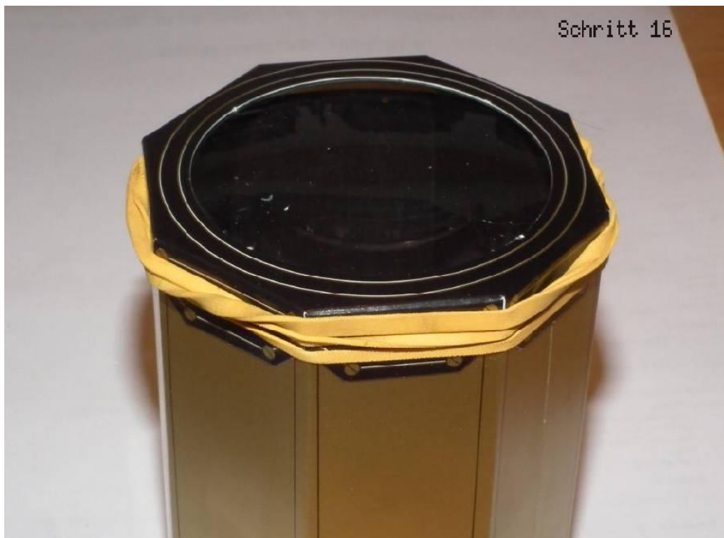
Step 16: The tabs of the lens holder are glued to the inner tube. A rubber band helps to keep the tabs in place until they dry.
