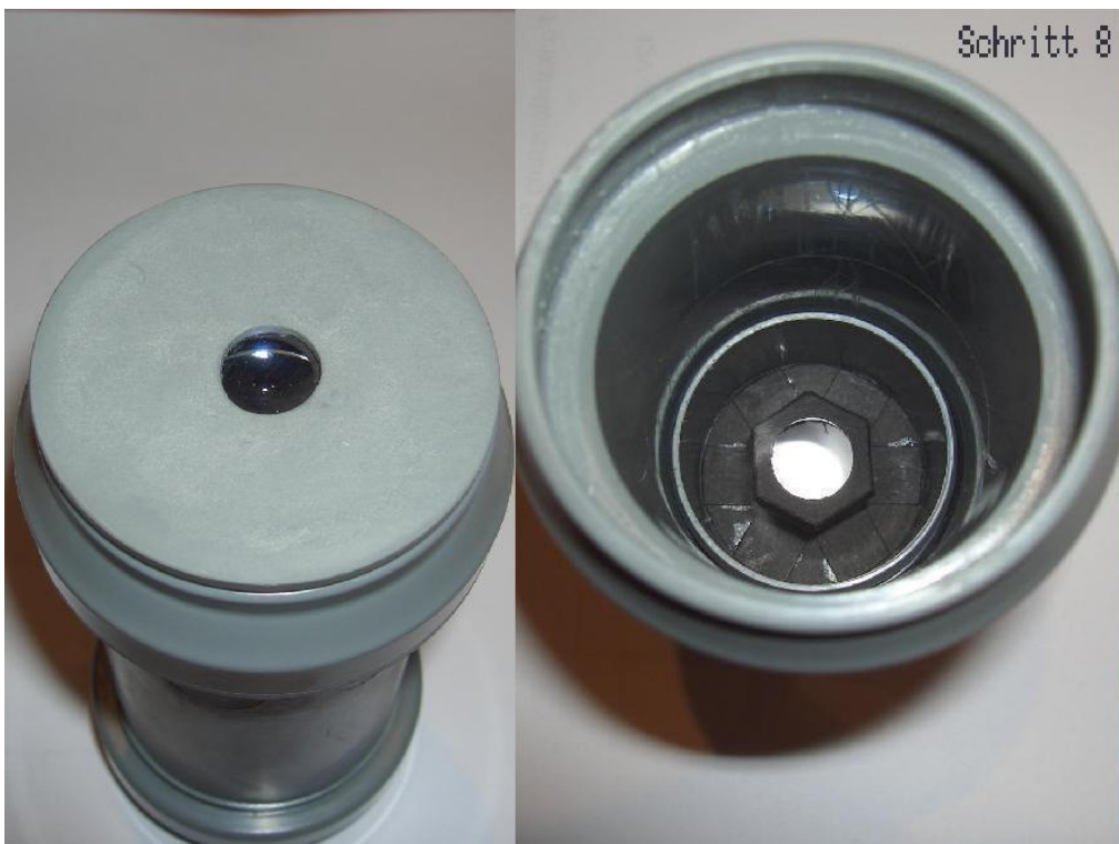
Step 8: Finished assembled eyepiece tube, inside and outside view.
